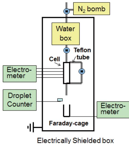
**Fig. 1** Experimental apparatus: (a) sandwich-type cell, (b) assembly.
