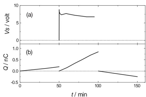
Fig. 4 Streaming potential (a) and charge accumulated in Faraday-cage (b) as a function of flow time. Cell material: quartz glass.
