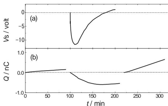
**Fig. 5** Streaming potential (a) and charge accumulated in Faraday-cage (b) as a function of flow time.
