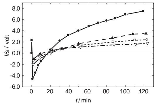
**Fig. 2** Streaming potential  $V_s$  as a function of flow time:  $\bullet V_{S(A-D)}$ ,  $\blacktriangle V_{S(C-D)}$ ,  $\circ V_{S(B-C)}$ ,  $\nabla V_{S(A-B)}$ . Cell material: quartz glass.
