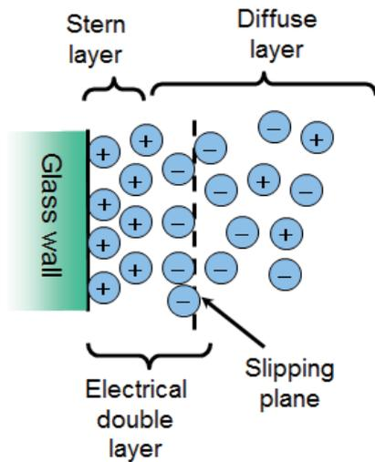
Fig. 3 Interface structure.
