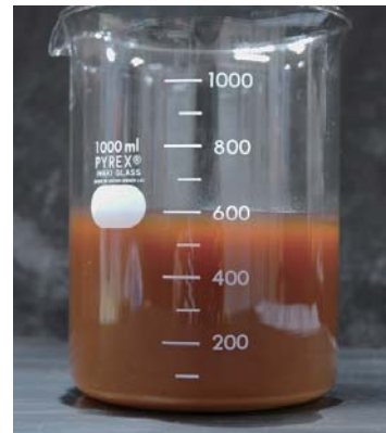
Fig.5 Representative photograph of emulsified A-Heavy oil (Water: 6 vol.% for Fuel, 800 rpm).
